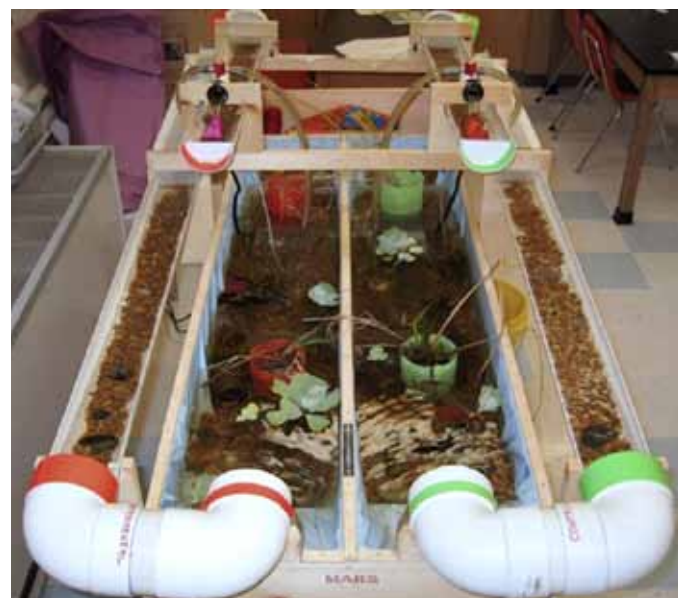
FIGURE 2. A more elaborate habitat, the Mobile Aquatic Research System (MARS) constructed by ScienceCorps Fellow Jon Letendre. "Control" and "Experimental" streams fed into separate ponds for side-by-side comparison of alterations following environmental stress.
