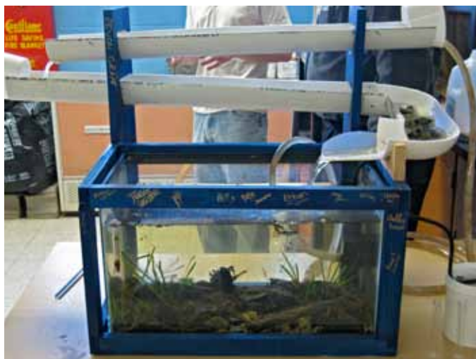
FIGURE 1. A simple "pond-and-stream" model system constructed by ScienceCorps Fellows Samuel Frankel and Melissa Hamel. Recirculating water through a PVC "stream" into an aquarium "pond" provided differential habitat for microbial and invertebrate life. Habitats provided a contextual framework for molecular investigation of macroscopic and microscopic organisms.
