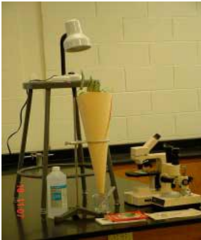
Experimental Setup: Berlese Funnel Apparatus
